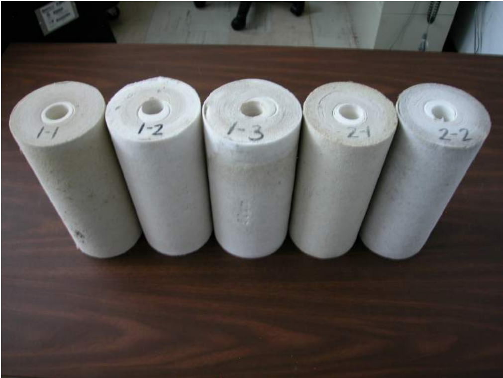
Side-by-side comparisons of scale build up on heaters (L-R: New, Control, SS, HF, and SS/HF)
