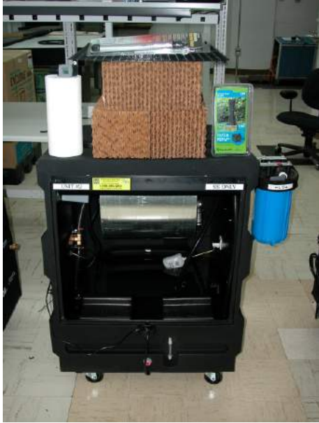
Figure 3. Unit #2 with Side-Stream Filtering Apparatus (50 micron filter)
