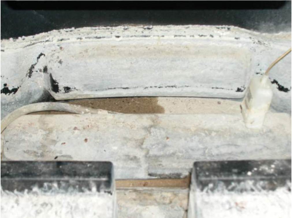
Post-test image of scale in Unit #3 basin
