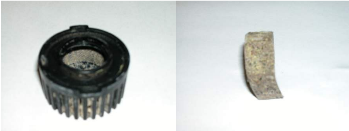
Figure 7. Debris and scale build-up on Unit #1 (control) pump filter July 22 nd pre-cleaning.
