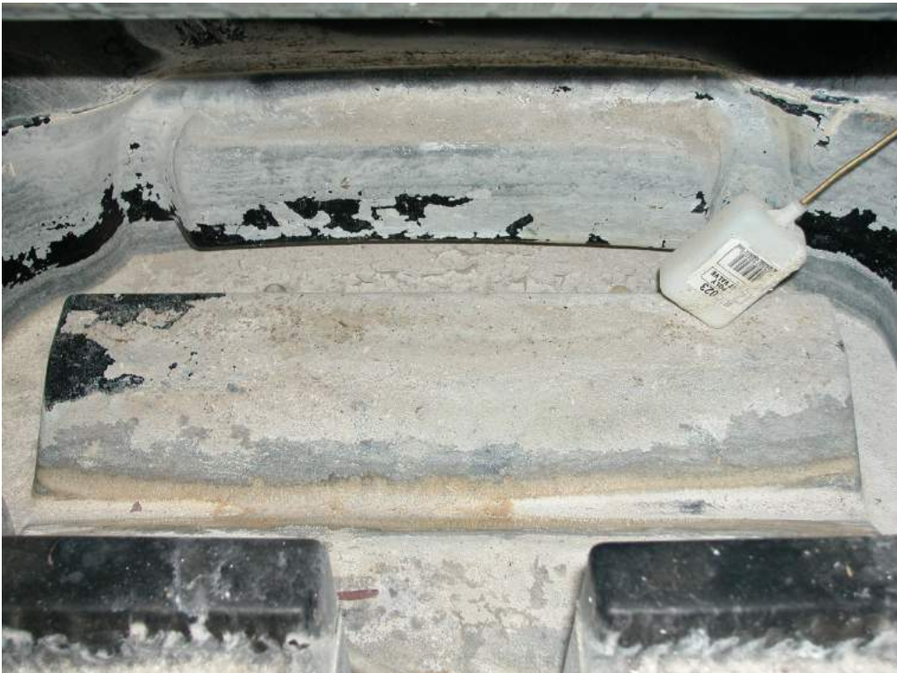
Post-test image of scale flaking in Unit #2 basin
