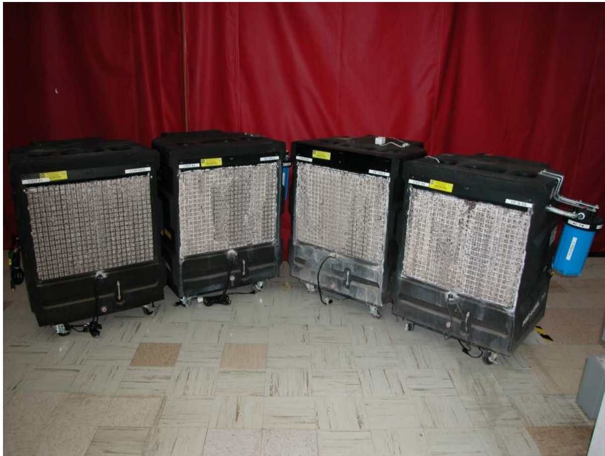
Figure 9. Post-test condition of evaporative coolers (L-R: Control, SS, HF, SS/HF).
