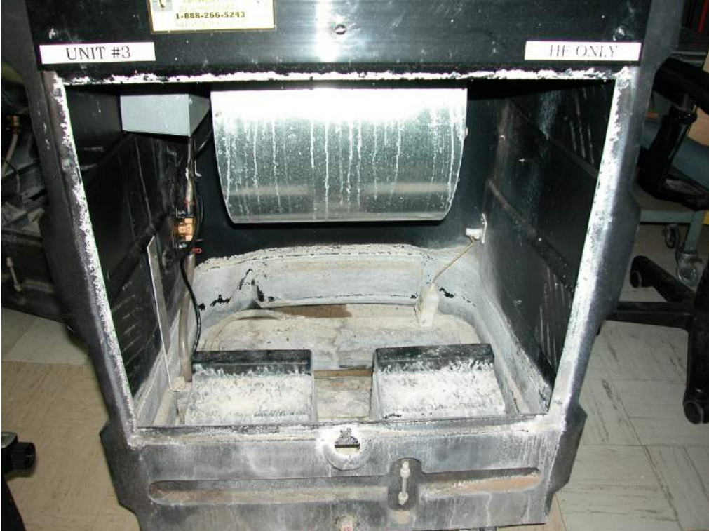
Post-test image of scale in Unit #3 basin
