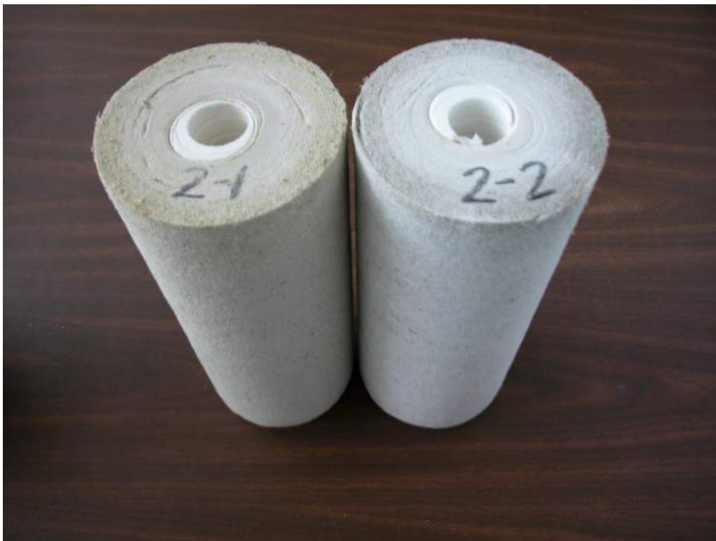
Post-test image of filters from Unit #4 (Side Stream w/ HydroFLOW)
