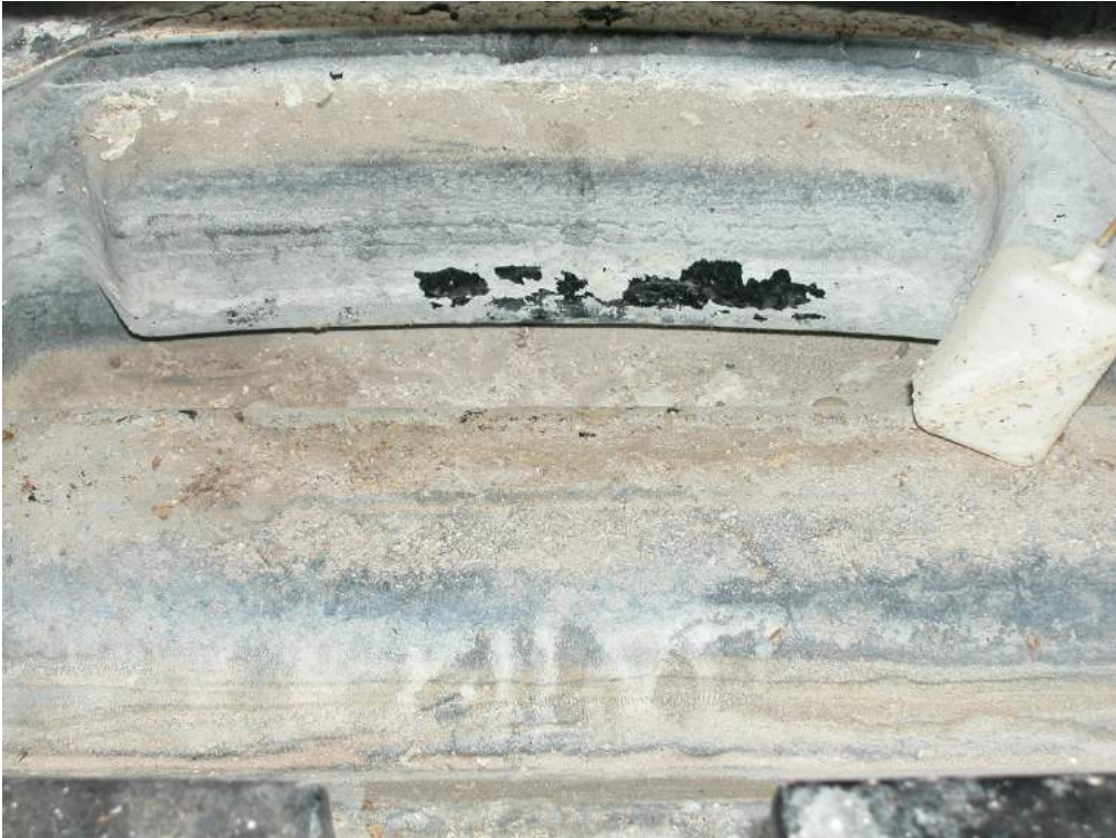
Post-test image of scale in Unit #4 basin
