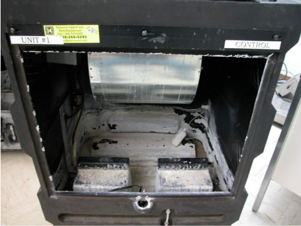
Post-test image of scale / sediment in Unit #1 basin
