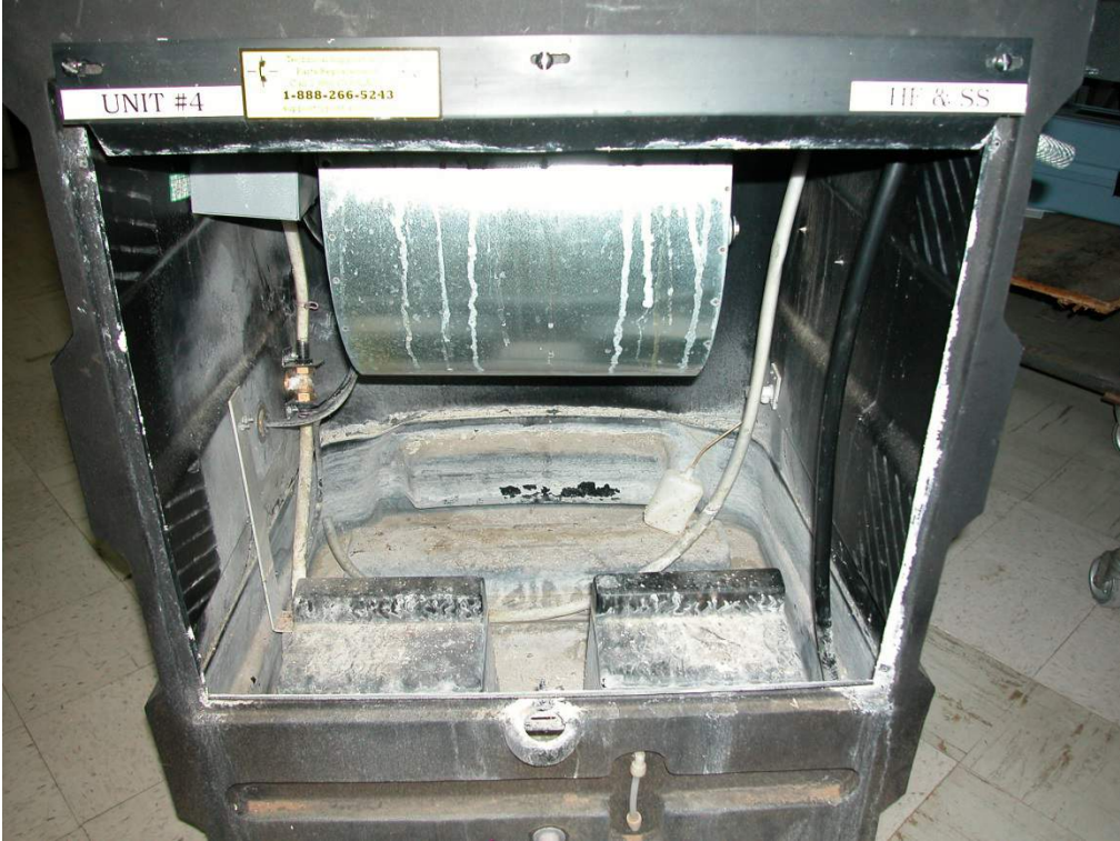
Post-test image of scale in Unit #4 basin
