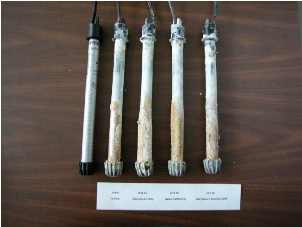
Side-by-side comparisons of scale build up on heaters (L-R: New, Control, SS, HF, and SS/HF)
