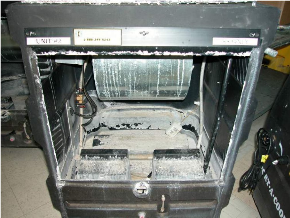
Post-test image of scale flaking in Unit #2 basin
