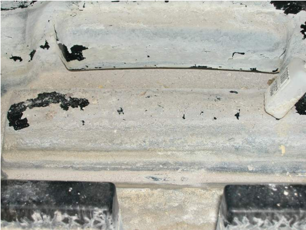
Post-test image of scale / sediment in Unit #1 basin
