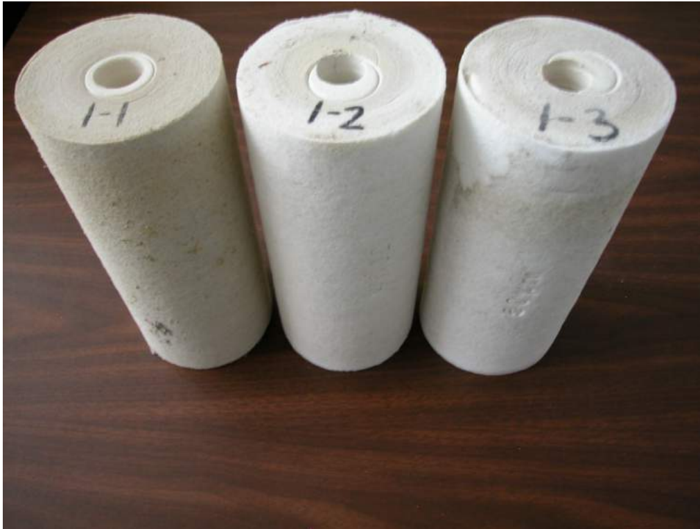
Post-test image of filters from Unit #4 (Side Stream w/ HydroFLOW)
