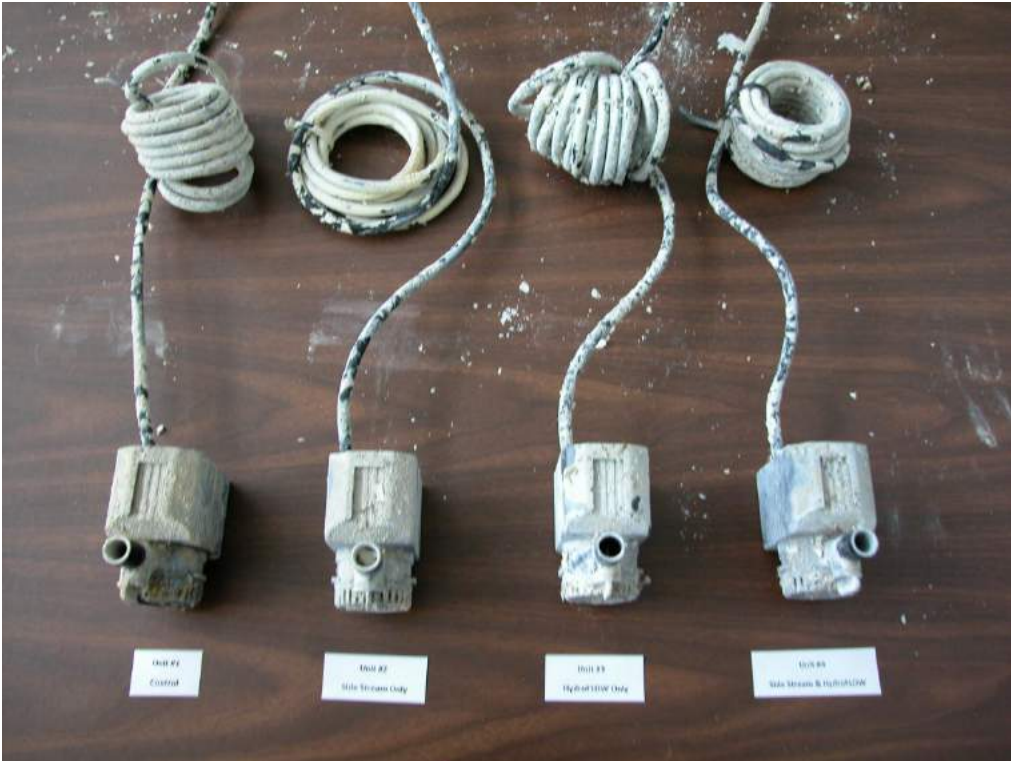
Post-test image of scale build up on recirculation pumps
