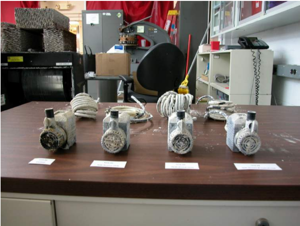
Post-test image of scale build up on recirculation pumps
