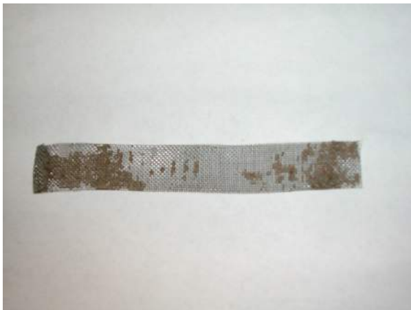
Figure 8. Scale build-up on pump filter to Unit #1 (post cleaning).
