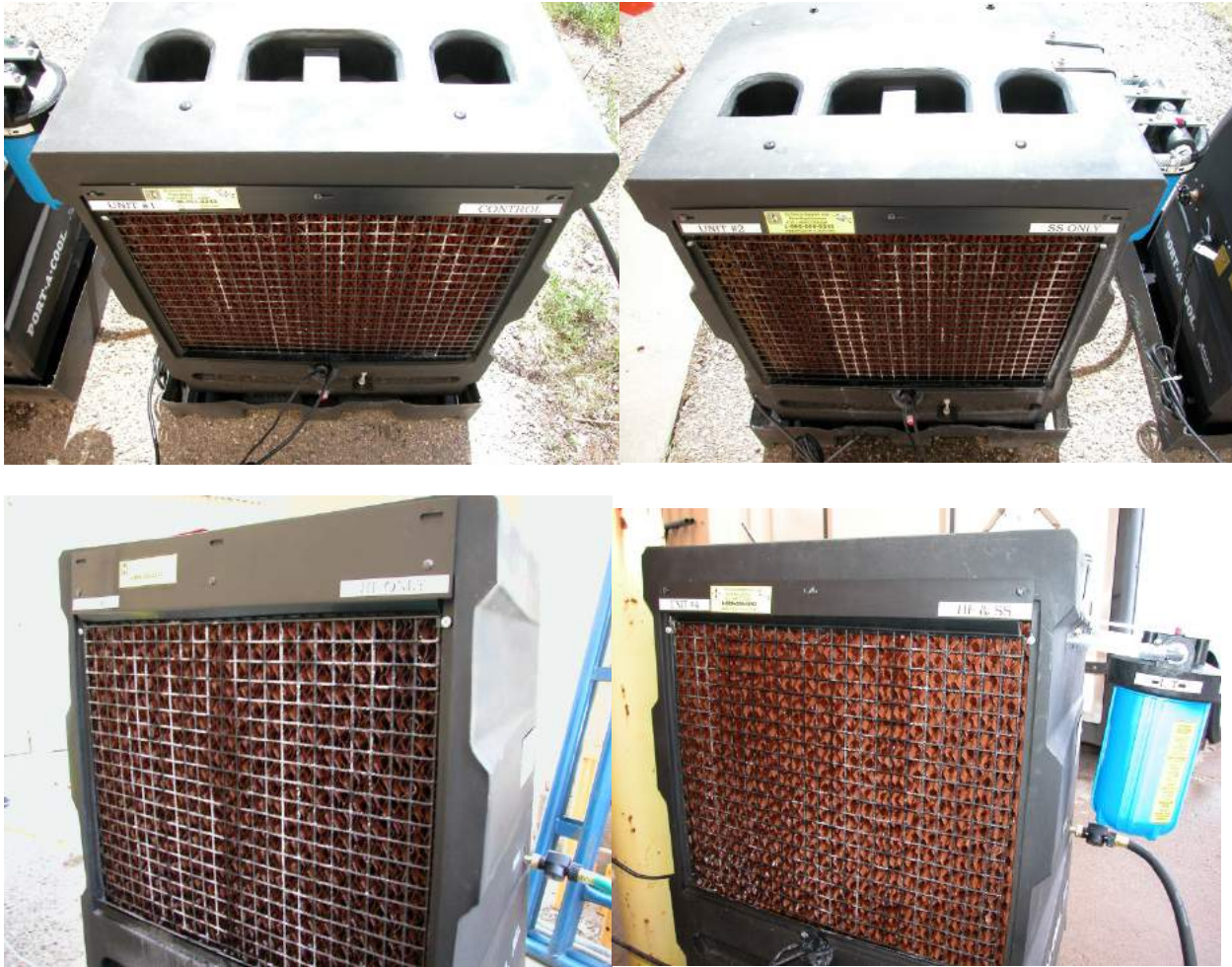
Figure 6. Scale build up on each unit being tested on May 26 th and 27 th . (top left) Unit #1 control, (top right) Unit #2 side-stream filtration only, (bottom left) Unit #3 HydroFLOW only, and (bottom right) Unit #4 side-stream and HydroFLOW.
